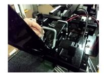
**Step 2:** Connect cannon plug from handle into the "J2" socket on speed control
