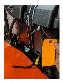
**Step 6:** Connect the male and female spade terminals from the handle to the corresponding terminals coming from the cylinder.
