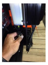
**Step 3:** Connect bullet terminal from handle to the wire coming from the parking brake
