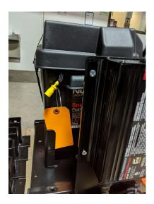
**Step 5:** Connect the yellow in line fuse holder(25A- red wire) and black with male bullet from the handle to the corresponding wire coming out the front of the battery box.
