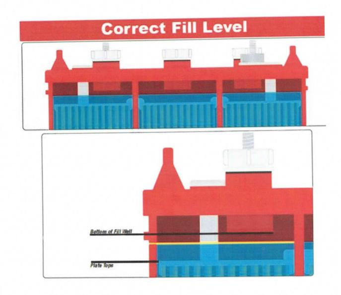
Caring for a flooded battery is as simple as topping up with water regularly to replenish the water which has evaporated. If this preventative maintenance is not conducted, the battery will deteriorate which can result in premature battery failure, or potentially an explosion.
