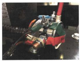
Attach the transmission cable to the handle as shown. Tighten the mounting nuts with an 11/16" wrench. Attach the socket at the end of the cable to the ball on the twist grip.
