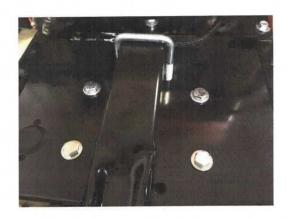
Tighten the washers/nuts from underneath.
