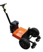
**Loading:** Position the ball of the tug under the receiver of the trailer and stop. Then either crank the trailer down onto the tug (Manual) or push the button to raise the ball up into the receiver and lift the tongue of the trailer up into the air (Automatic). Do not hold the button when the cylinder is maxed out on stroke. This can cause damage to the cylinder motor and electronic circuits.
