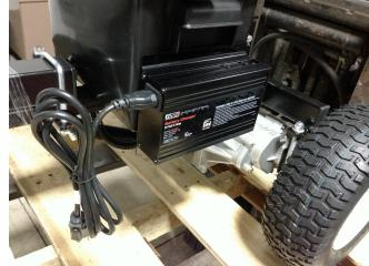
**Step 2:** If you purchased the "Surge Brake By-Pass", plug in the trailer electric to the plug on the tug labeled "Surge Brake By-Pass" and this will not allow the brakes to lock up when pushing the trailer in reverse.
