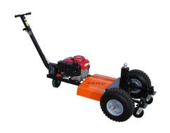
**WARNING:** This tug is shipped WITHOUT gas or oil in the engine. Using the 10W-30 Oil provided, fill to the "Full" mark on the dipstick. Fill the fuel tank with regular unleaded gasoline (Non ethanol). Refer to engine manual for additional information.
