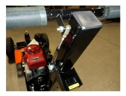
Then open the nuts located several inches from the hand grip on the cable and slip the cable between the bracket on the left side of the handle and then secure the nuts firmly using an 11/16" wrench.
