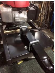
**Step 2:** Attach the transmission cable end to the left hand grip with the "ball" on it. Then open the nuts located several inches from the hand grip on the cable and slip the cable between the bracket on the left side of the handle and then secure the nuts firmly using an 11/16" wrench.
