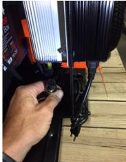
**Step 4:** Connect red wire with fuse holder from the handle to the mating fuse holder on the side of the batteries
