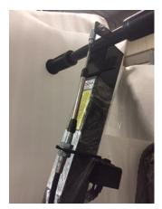
**WHEELIE BARS:** Wheelie Bars are located on the back of the tug to prevent the tug from tipping in extreme circumstances (i.e. starting too quickly or stopping too abruptly).
