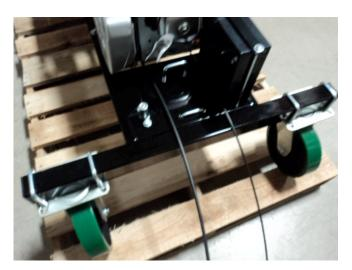
**Step 2:** Install the handle all the way through second "U" bolt. Push the handle approximately 1 1/2" beyond the second "U" bolt. If it appears the handle will not fit through the "U" bolt, loosen the nuts below. Once the handle is installed, tighten nuts securely.
