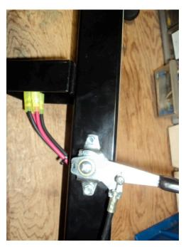
**Step 4:** Connect the transmission cable end to the left hand grip with the "ball" on it. Then open the nuts located several inches from the hand grip on the cable and slip the cable between the bracket on the left side of the handle and then secure the nuts firmly using an 11/16" wrench.
