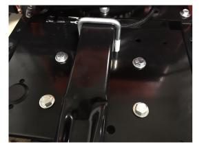
Tighten the washers/nuts from underneath.
