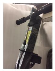
**WHEELIE BARS:** Wheelie Bars are located on the back of the tug to prevent the tug from lifting the handle in extreme circumstances (i.e. starting too quickly or stopping too abruptly).
