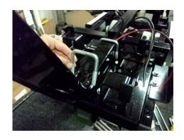
**Step 2:** Attach the transmission cable to the handle as shown. Tighten the mounting nuts with an 11/16" wrench. Attach the socket at the end of the cable to the ball on the twist grip. Then attach the wires coming out of the bottom of the handle to the battery leads(quick disconnects). Lastly run the longer two wires under the right side of the engine and connect them to the mating connections coming from the cylinder.
