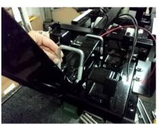
**Step 2:** Attach the transmission cable to the handle as shown. Tighten the mounting nuts with an 11/16" wrench. Attach the socket at the end of the cable to the ball on the twist grip.
